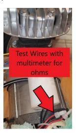
8. Check Power going to AC Pump Connection
