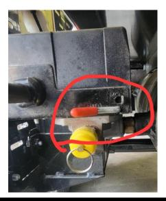
These connections can come loose in the shipping/delivery process. There will be zip ties on the white connections, but that doesn't mean the connections are good.
