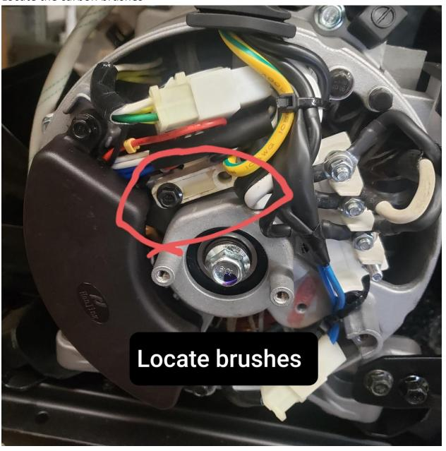
3. Make sure both connections are firmly connected by removing them both off the brushes. Make sure there is no debris on the contacts of brushes and connections to wires are good. Reconnect and try generator power output again.
